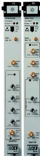
Figure 16 13.5 Gbit/s Generator and Analyzer Modules
