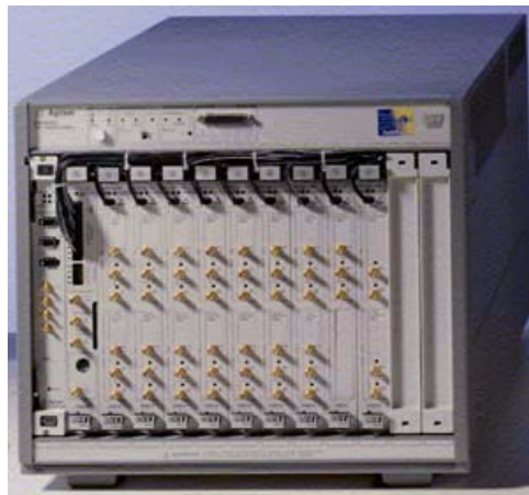
Figure 3 VXI Mainframe with IEEE 1394 Interface and Modules
