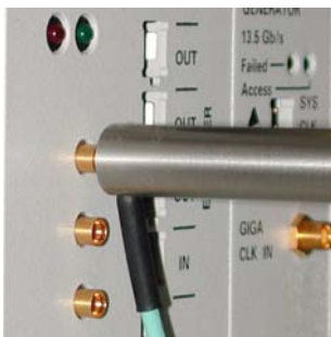
Figure 322 Use the Plug-In Tool to Insert the Cable Connector
