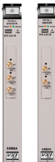
Figure 11 E4866A/E4867A 10.8 Gbit/s Data Generator/Analyzer Modules
